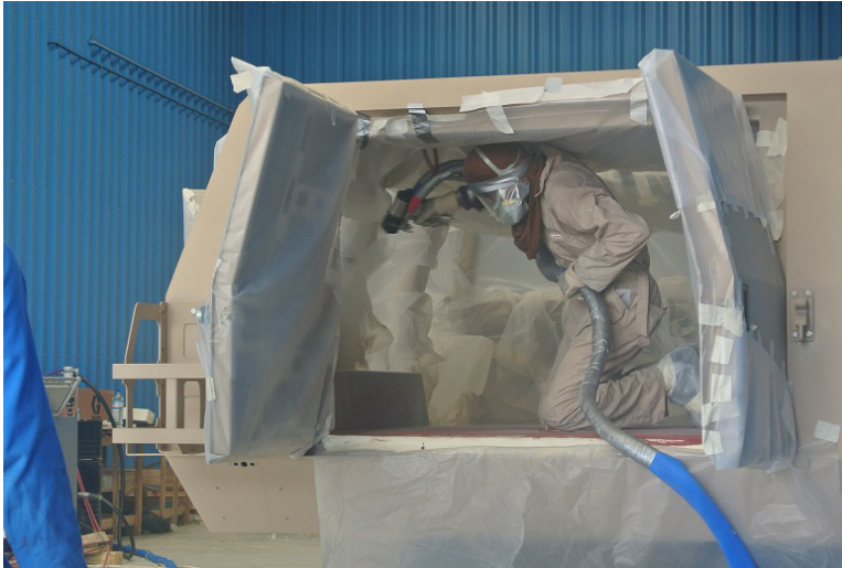
Armored car – inside protective coating
